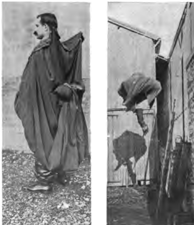
A LIFE PRESERVING GARMENT FOR AVIATORS, WHICH FORMS INTO A PARACHUTE ON FALLING.
